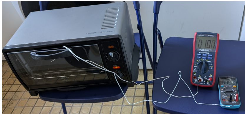
Figure 13: High-temperature testing setup
